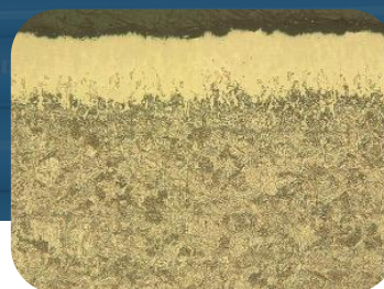
Microstructure of boride layer below ID bore surface
